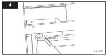
TAKE EXTREME CARE WHILST REMOVING THESE PANELS NOT TO SCRATCH OR CHIP THE PANEL ON THE SIDES OF THE FIREBOX.
